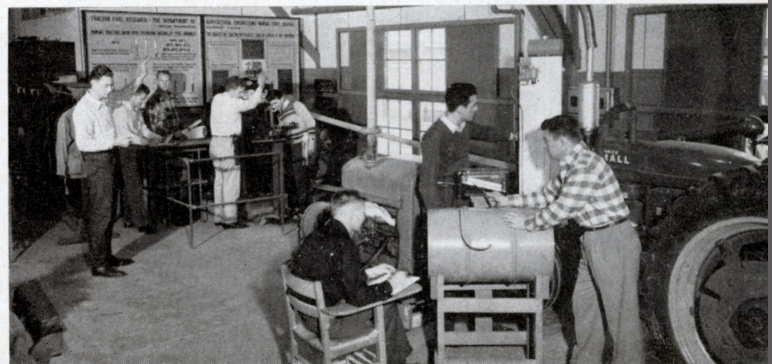
Agricultural Engineering students in a Farm Motors Laboratory class checking the performance of a farm tractor by measuring brake horsepower, and fuel and air consumption.
